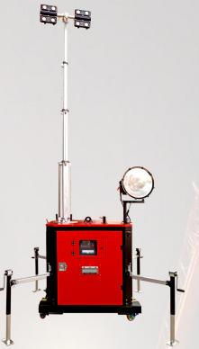
**Brief specifications** Minimum dimensions(L\*W\*H) 1540\*1540\*1800mm Maximum dimensions(L\*W\*H) 2380\*2380\*5380mm 900kg Dry weight Lifting system Electric 179° Mast rotation 2\*350W Lamps power LED Lamps type Total lumen 16730 Lm Illuminated area 4500 m<sup>2</sup> Engine Battrey Outlet socket (KVA/V/Hz) 2, 5/220/50-2, 5/240/60 16/220/50-16/240/60 Inlet plug (A/V/Hz) 80 km/h Wind speed resistance Running time 10 h
